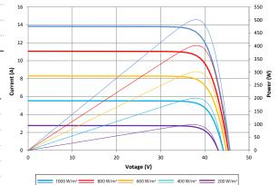
Current-Voltage & Power-Voltage Curve (500S)
