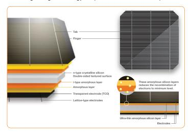
Advanced bifacial cell designed for increased energy output. The cell utilizes sunlight reflected back from the rear side material which captures more light and converted into energy.
